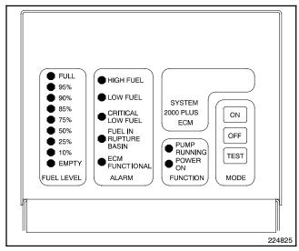
Figure 3-2 ECM Front Panel Layout
